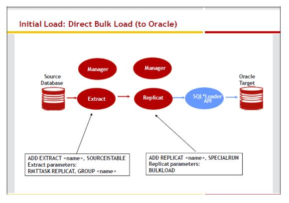
The Replicat process will be automatically started by the Manager process. The port used by the Replicat process may be controlled using the DYNAMICPORTLIST Manager parameter.
