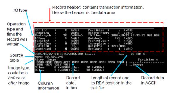
GoldenGate trail files are unstructured. The GoldenGate record header provides metadata of the data contained in the record and includes the following information.
